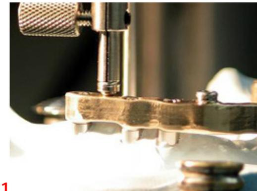
3. Tack the Laser Bar Female into place on top of the bar by placing a spot of laser weld on opposite sides of the female (**FIG 2**).
